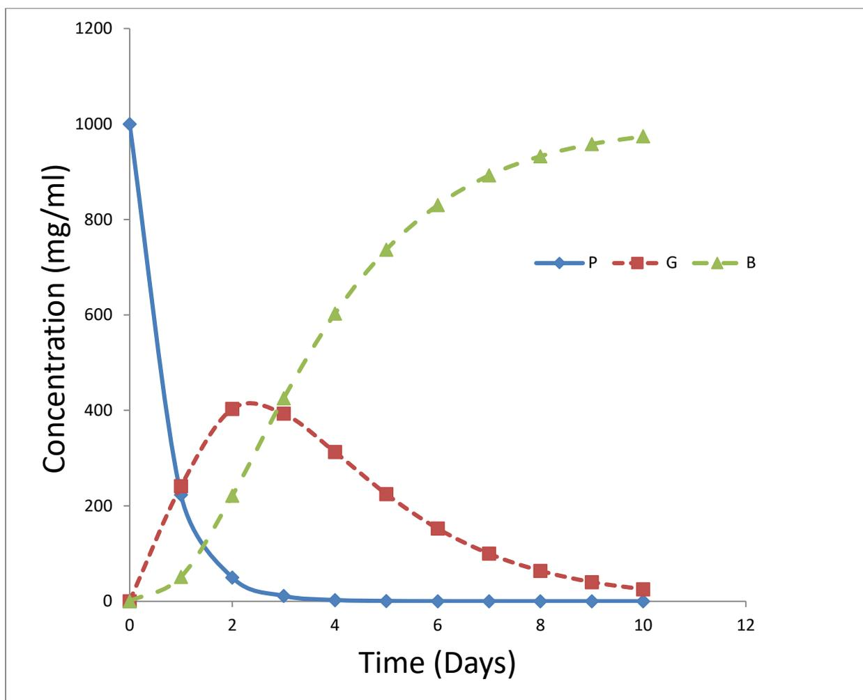
**Figure 4: A Plot of the Rate of Change of Unpretreated Plantain Trunk Biomass, Glucose Yield and Butanol Produced with Time**
