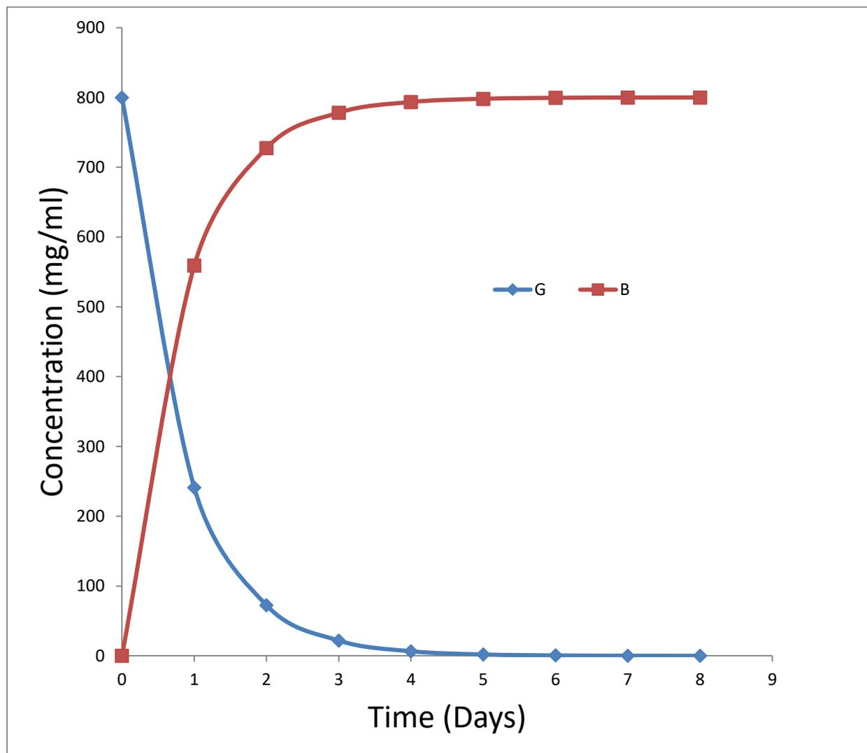
**Figure 3: A Plot of the Rate of Change of Glucose Concentration and Butanol Yield with Time**
