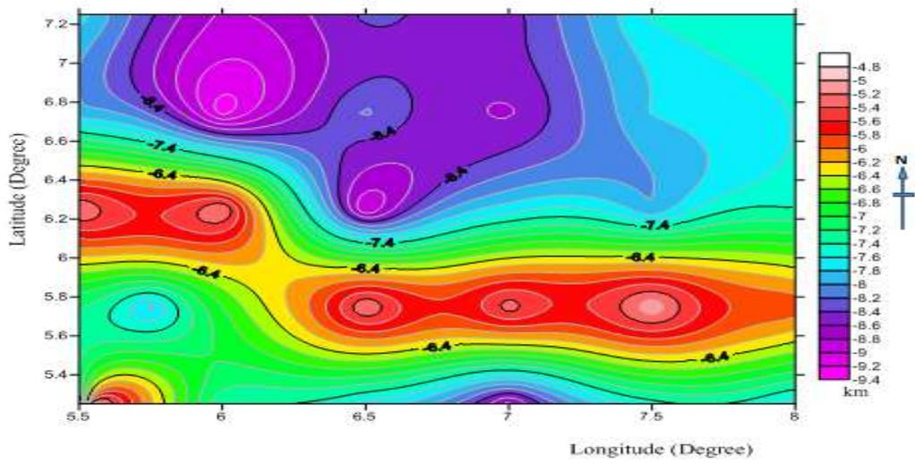
**Figure 2.2: The basement depth map obtained from spectral analysis for the study area**
