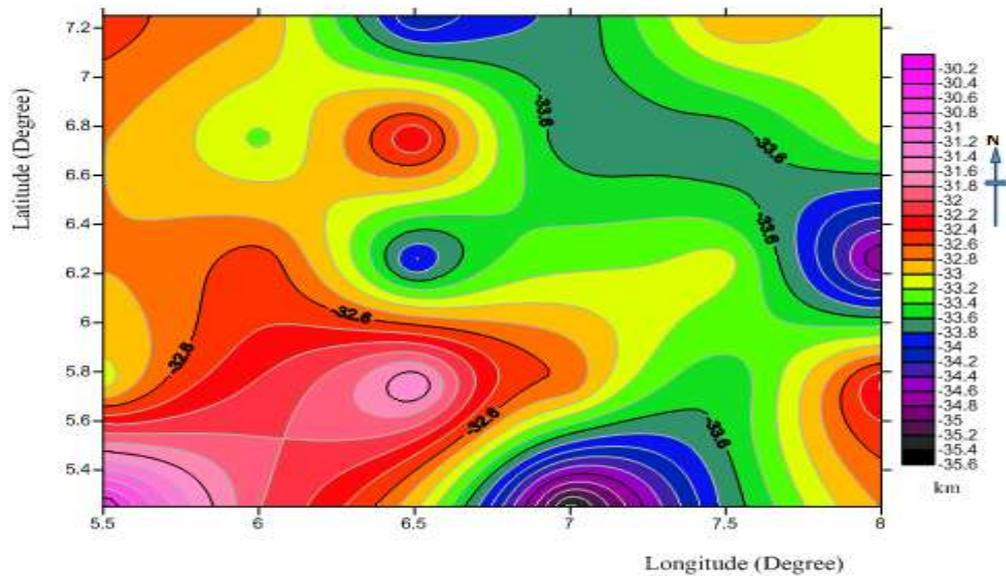
**Figure 2.4: Contour map of the crustal thickness obtained from spectral analysis of the study area**
